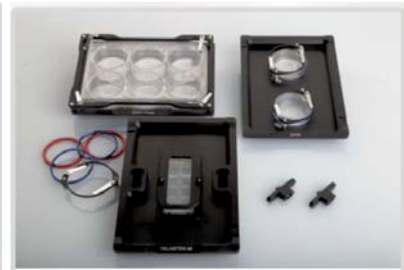
Example of Okolab incubation chamber or heating stage insert with CO 2 control option
