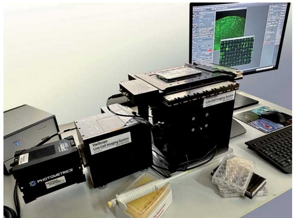
VisiScope Cell Analyzer based on ZABER MVR microscope and Crest CICERO Spinning Disk Confocal
