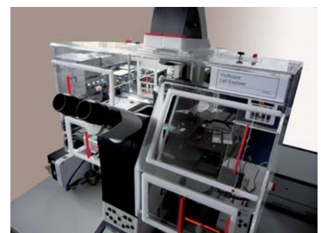
VisiScope Cell Analyzer based on Leica DMI microscope
