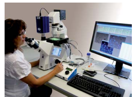
VisiScope Cell Analyzer based on Zeiss Axio-Observer microscope
